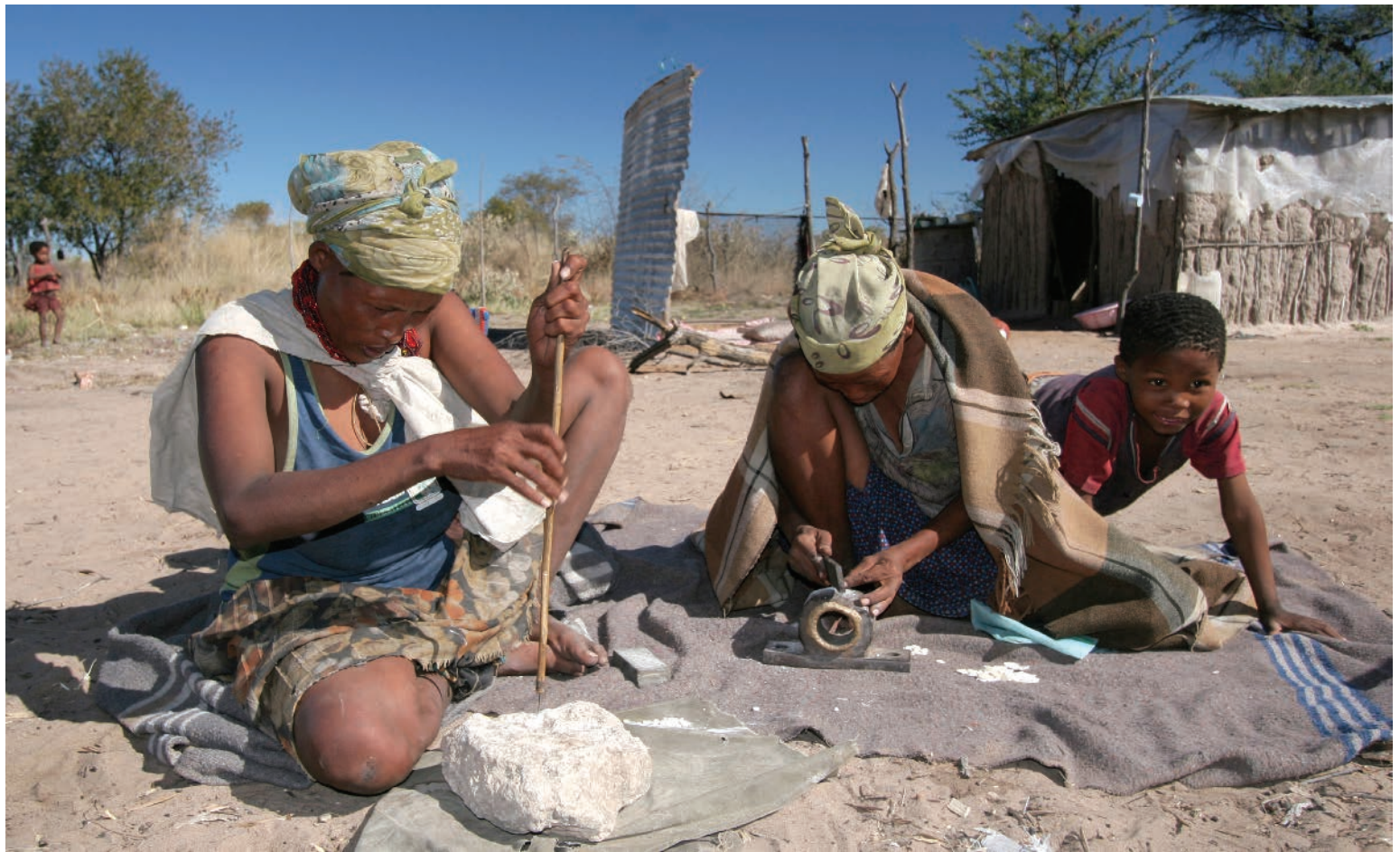
Figure 5: Traditional OESB: breaking shells into small fragments (right) before drilling holes with a metal nail (left).
