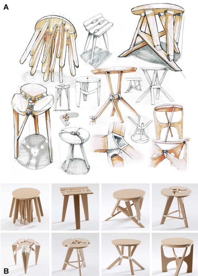
Figure 7 Concept designs, sketches, and investigations. (A) Initial sketches of concept designs for hybrid stools that require Digital Joinery for construction, and (B) several 3D-printed miniature stools to evaluate design ideas.
