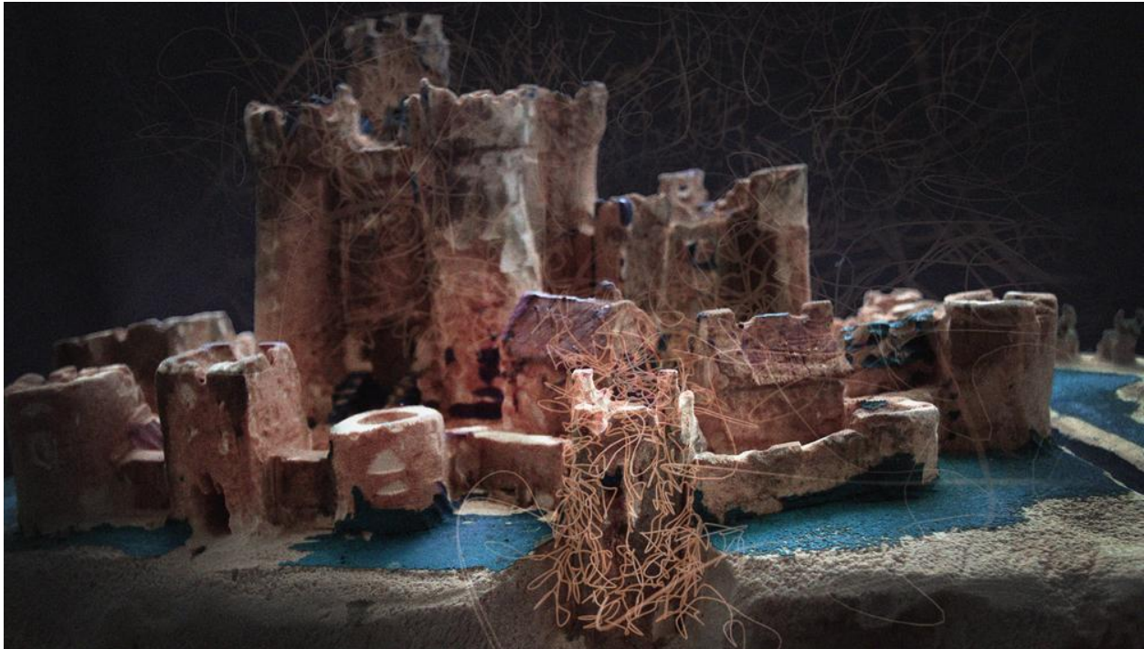
Figure 6: Unification in differences ---a castle model fabricated using the FreeD, and the tool path of the device used by the author in making this castle. Rendering by Rhino and VRay, and Photoshop editing. (© Amit Raphael Zoran)
