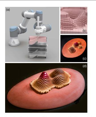
**Fig. 4.** (a) Illustration of a robot arm modifying a programmable silicon mold. (b) Mold. (c) and (d) Two versions of a mousse dessert, exemplifying the potential of the modular mold.
