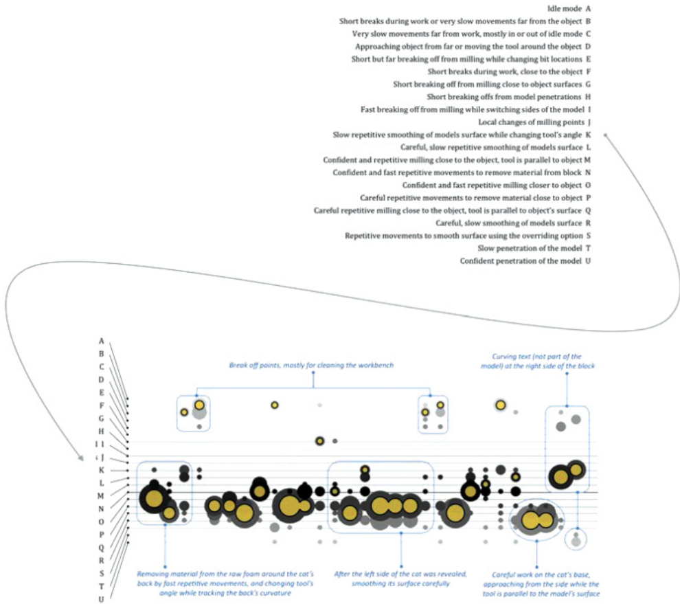
Fig. 16. Twenty-one different techniques (A–U), with Peter’s tool path for demonstration, where the timeline is constructed by averaging over time windows of 2.5 minutes. The size of the bubbles represents the relative time in that state at a given time point, while the yellow mark represents the dominant technique.
