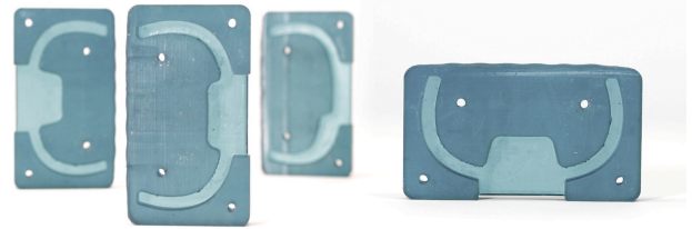
Figure 4 3D-printed plastic molds made by stereolithography for silicone casting of the 27 rib-molds.
