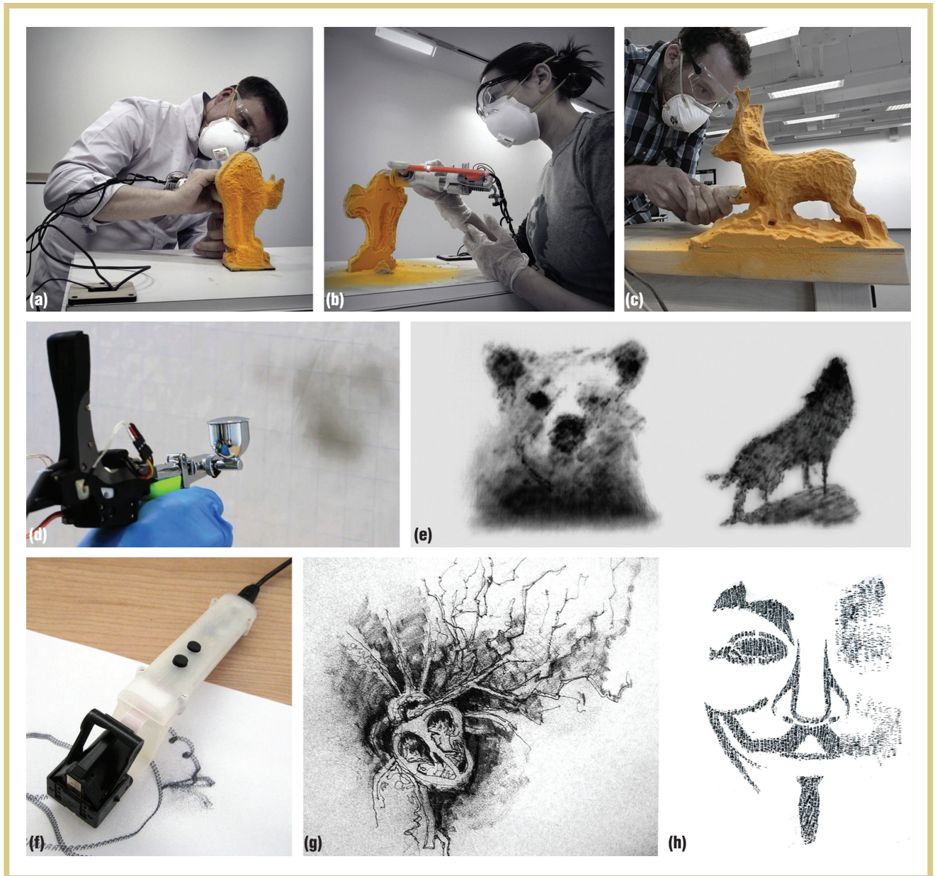
Figure 6. Smart tools in action. (a) Using FreeD in balsa foam to create a model of a cat. (b) Another user creating the same model of a cat. (c) A user works on a deer project involving six makers. (d) An early test of our smart airbrush and initial results of its use painting (e) a bear's face and a wolf. (f) Marcelo Coelho's BitBrush tool and (h) an example of artwork produced using it. (g) Artwork produced using the tracked version of Nishanchi.
