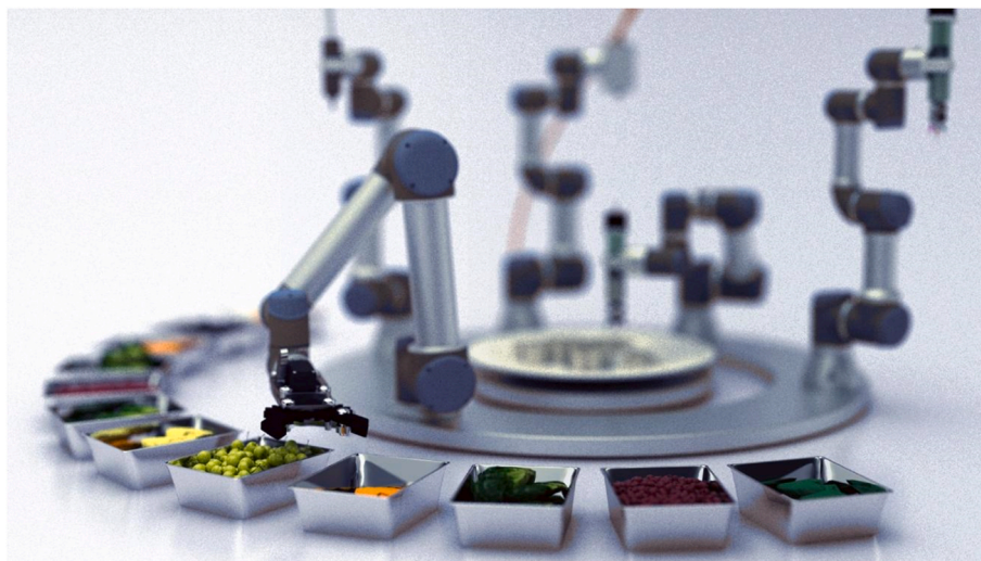
Fig. 9. Illustration of robotic arms working in synergy—printing, heating, scanning and precisely positioning and assembling a dish from ready-made elements.
