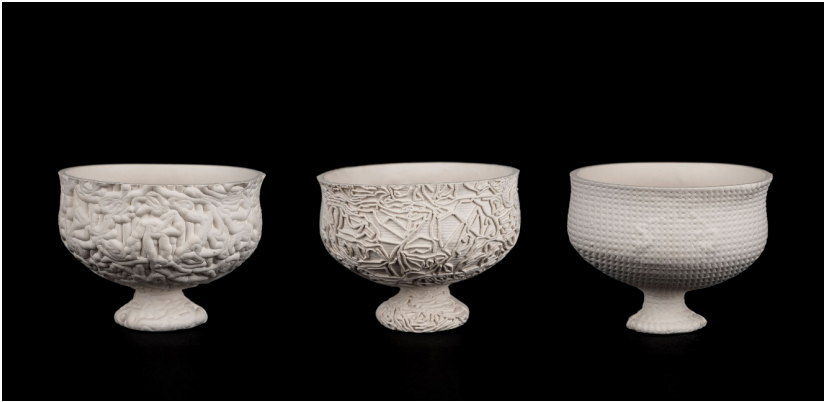
Fig. 2. Various versions of Kylix . Right, standard parallel finish. Middle, surface decoration by a mesh-derived toolpath and a sharp conic cutting tool. Left, the same toolpath using a 1/4-inch ball-nose cutter. (Photograph ©Asaf Oren)
