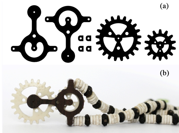
Figure 12: Design of a working gear mechanism (a), and the final assembly of the jewelry (b). We designed the gear-pendant and Ju/'hoansi integrated our work inside the necklace.
